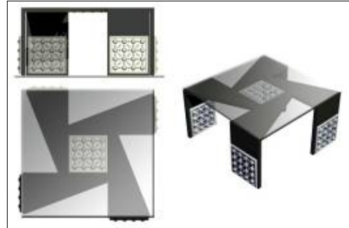
Figure (31, 32) Contemporary coffee tables using 3d printed Mashrabiya units- the researcher design
