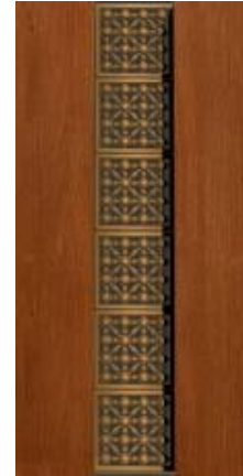
Figure (30) 3d printed Mashrabiya units of polyamide used in partition between interior spaces - The researcher design
